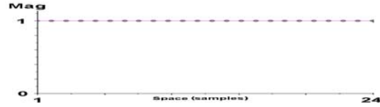
Figure 6: Space domain response after inverse Fourier transformation of Figure 5. Comparing with Figure 3 shows that desired samples are properly extrapolated.
