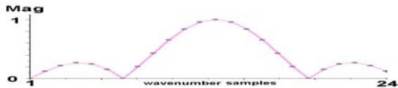
Figure 4: Wavenumber response of the event given in Figure 3. This is a sinc function.
