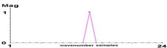
Figure 5: Wavenumber response after sharpening. Here all samples except peak sample are simply zeroed to illustrate the concept.
